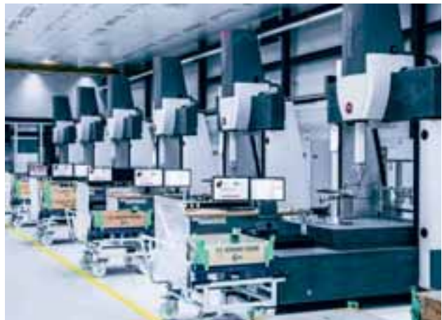
Better than the human eye _____ The quality assurance processes in the blisk manufacturing facility are supported by computer-controlled optical measuring systems.
