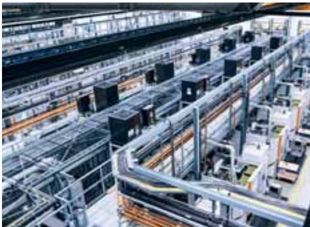
Automated loading _____ In MTU’s blisk production center in Munich, raw components are routed directly to the machines, which adjust their settings accordingly.
