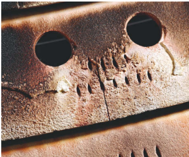
Delamination _____ Damage to the thermal barrier coating in the combustion chamber of a CF6-80C2.
