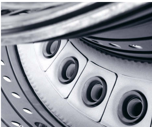
Restored _____ CF6-80C2 combustion chamber with thermal barrier coating.
