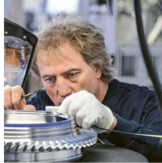
A PW1100G-JM high-pressure compressor blisk is masked prior to plasma spraying.
