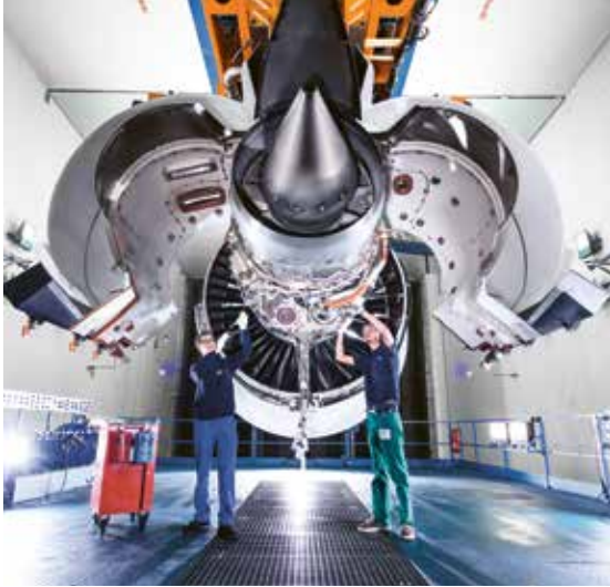
A PW1100G-JM in the test cell at MTU Maintenance Hannover. These engines power the A320neo aircraft family.
