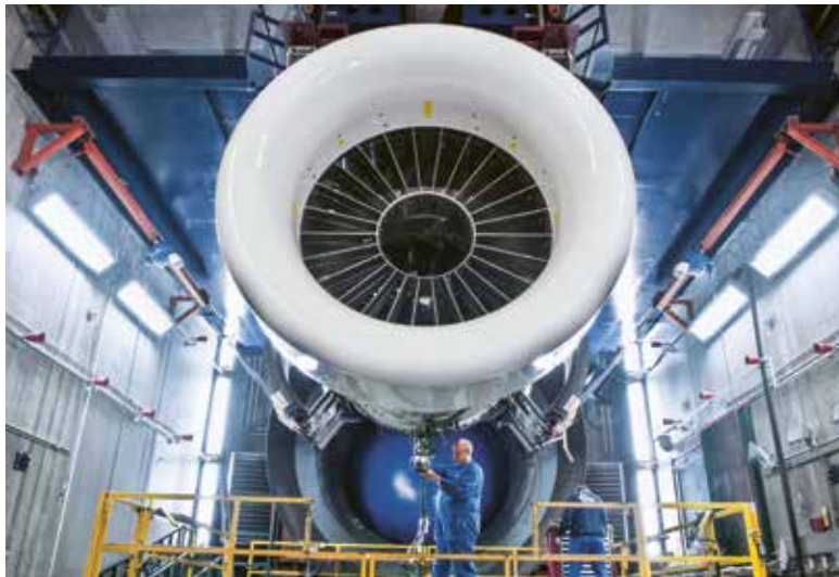
A PW1500G powerplant for the Bombardier C Series in the test cell at MTU in Munich.
