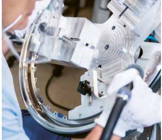
Component production _____ A V2500 ring is deburred at MTU Aero Engines Polska.
