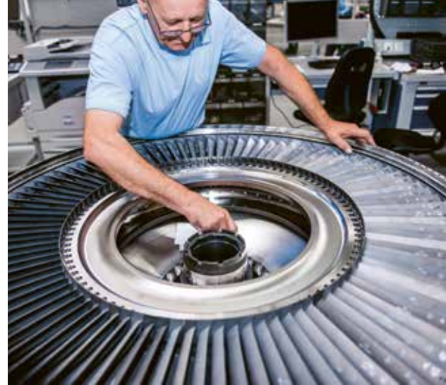
Module assembly _____ A PW2000 low-pressure turbine is assembled at MTU Aero Engines Polska.
