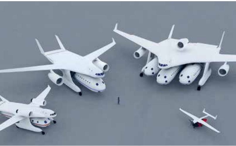
Versatile — The Clip-Air concept is based on interchangeable modules of different sizes for carrying freight, passengers or fuel, depending on demand.
