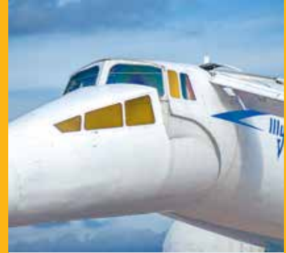
Droop nose — Both the Concorde and the Tupolev Tu-144 featured a nose cone that pilots could lower to improve visibility on the ground.
