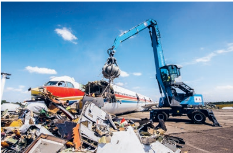
Aircraft recycling — Heavy machinery and equipment is required to dismantle an aircraft. Removal of potential replacement parts like engines and landing gear must be done by experts. Following the prep work, it takes between two and six days to disassemble an aircraft, depending on its size.
