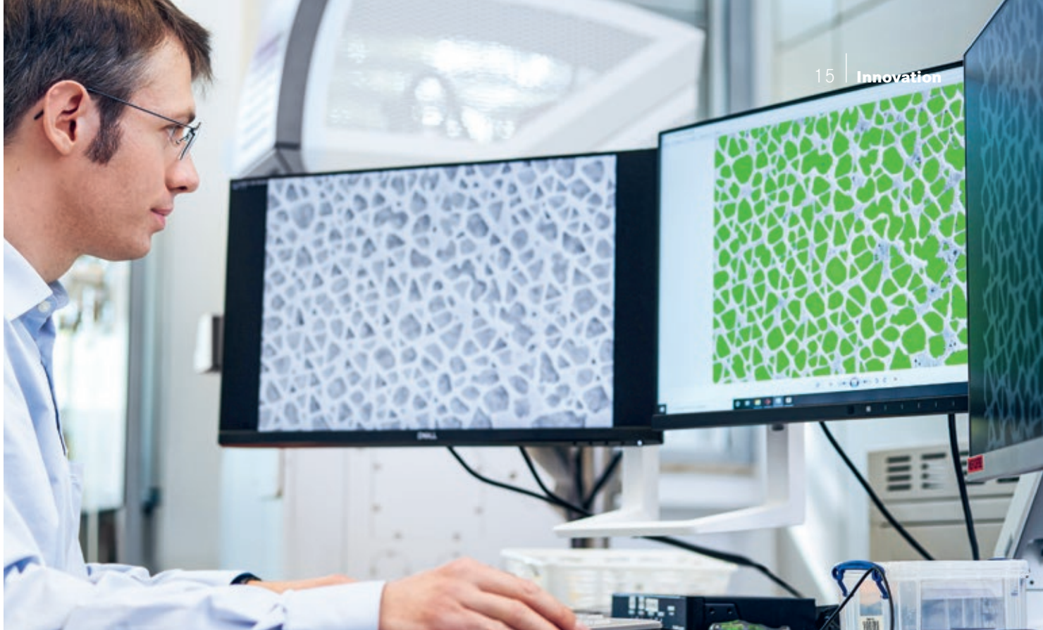
Automated image analysis — Natter adds color to one phase of the material. This serves to classify material properties to assess factors such as overheating of the material during flight.
