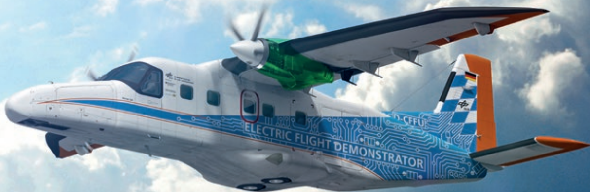
Dornier 228 — The twin-engine turboprop aircraft will be equipped with a hydrogen-powered fuel cell and used as a flying testbed.
