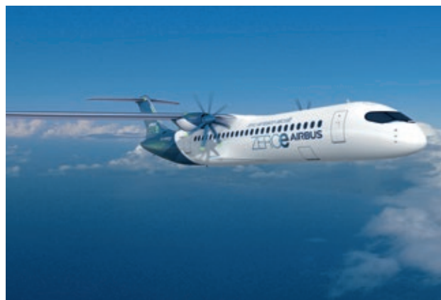
Turboprop design — The aircraft for up to 100 passengers has a range of more than 1,000 nautical miles.
