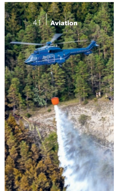
Airbus Super Puma ____ Operated by the German Federal Police, this helicopter can hold 2,000 liters of water.
