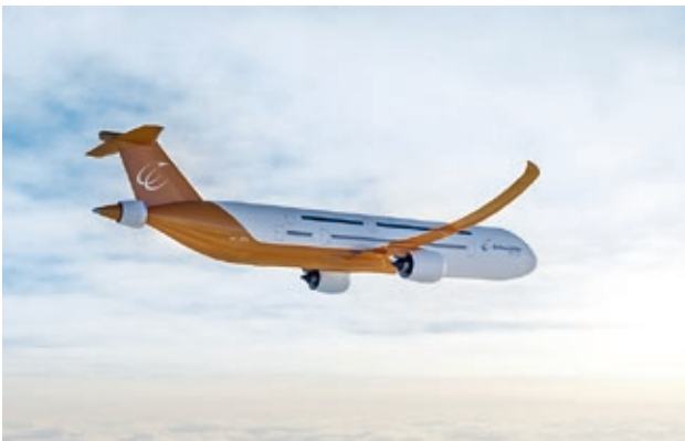
Propulsive fuselage — The enlarged fuselage surface of a hydrogen aircraft results in synergetic savings potential when using a propulsive fuselage.
