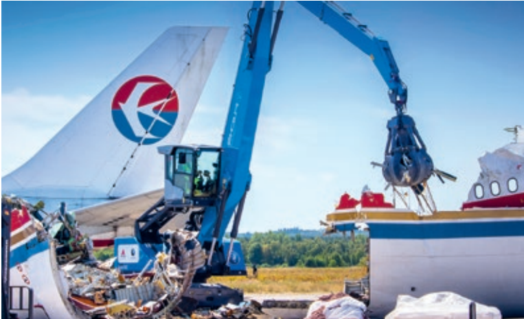
Aircraft recycling — Heavy machinery and equipment is required to dismantle an aircraft. Removal of potential replacement parts like engines and landing gear must be done by experts. Following the prep work, it takes between two and six days to disassemble an aircraft, depending on its size.
