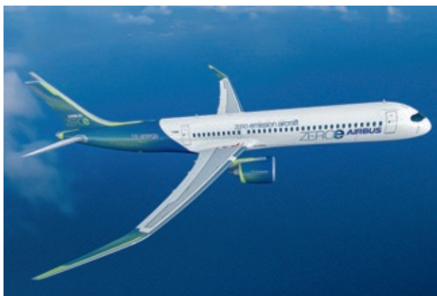
Turbofan design — The aircraft for 120 to 200 passengers has a range of more than 2,000 nautical miles.
