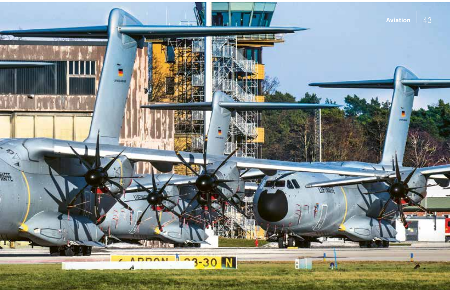
The most powerful turboprop in the West — Four propellers with an impressive diameter of 5.33 meters power the transporter.
