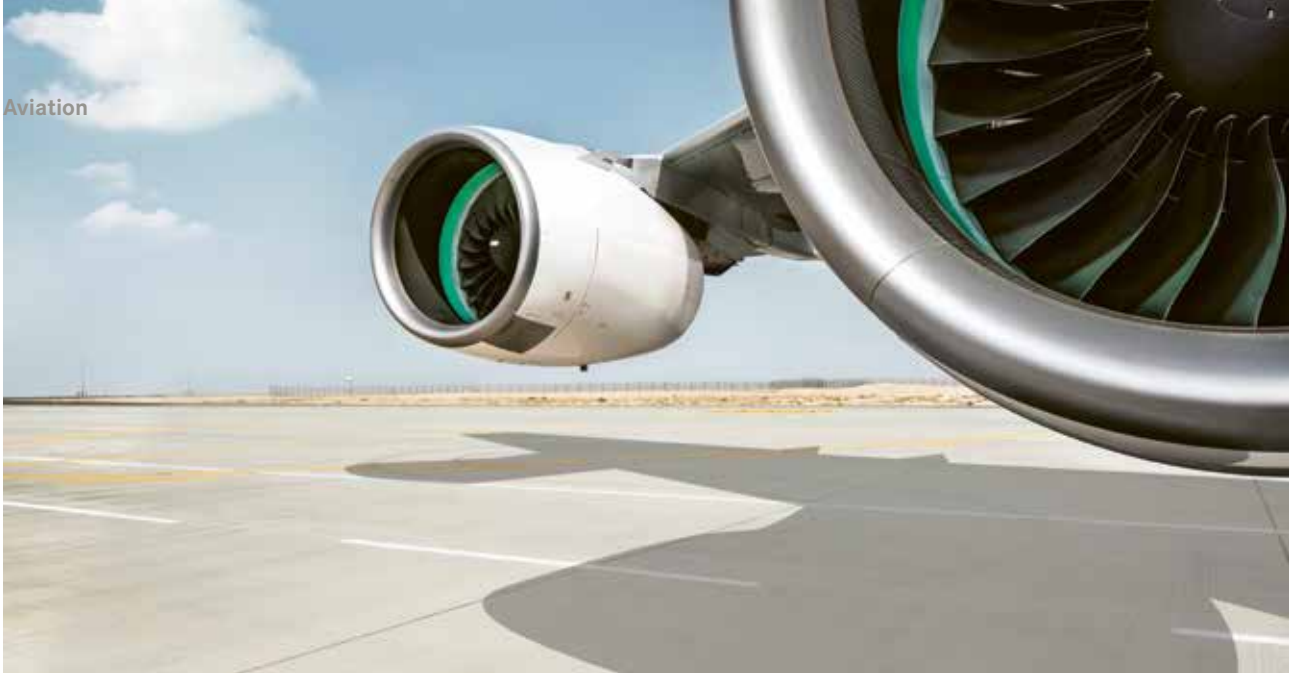
Technology from two worlds — The GP7000 is based on proven engine technologies from GE Aviation and Pratt & Whitney, which the two companies pool together in their Engine Alliance joint venture.
