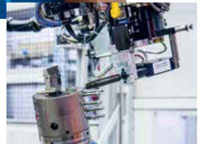
Automated manufacturing — MTU manufactures some of its high-pressure turbine airfoils fully automatically.
