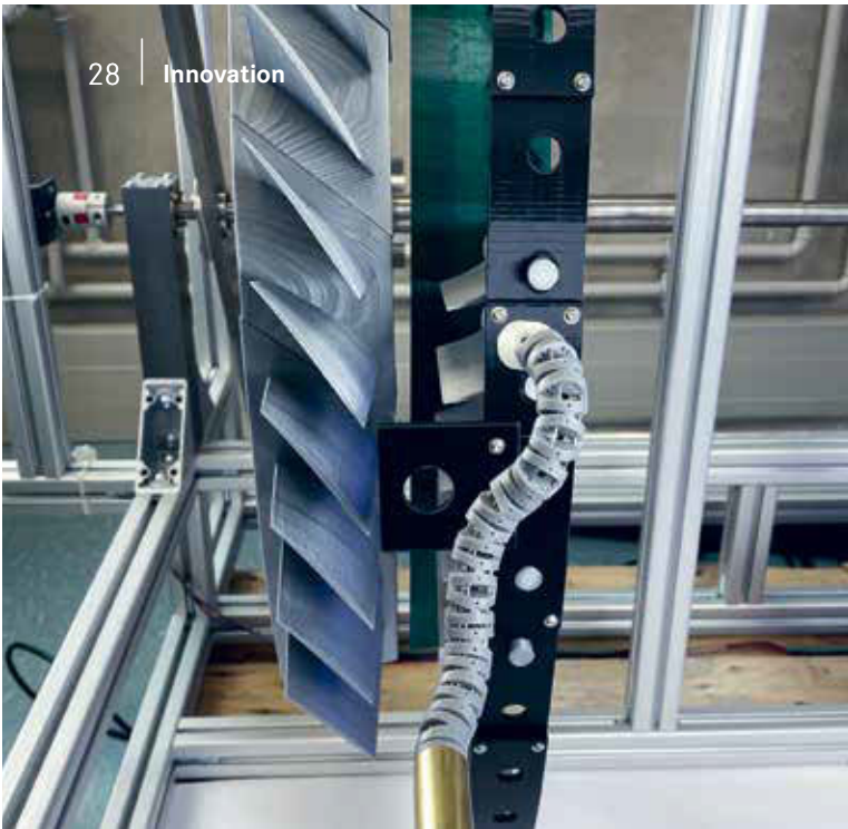
Research on a laboratory scale — Running experiments with the RoBokop on a stage of a high-pressure compressor. The model has been scaled up by a factor of 2.5 to make conducting the experiments easier.
