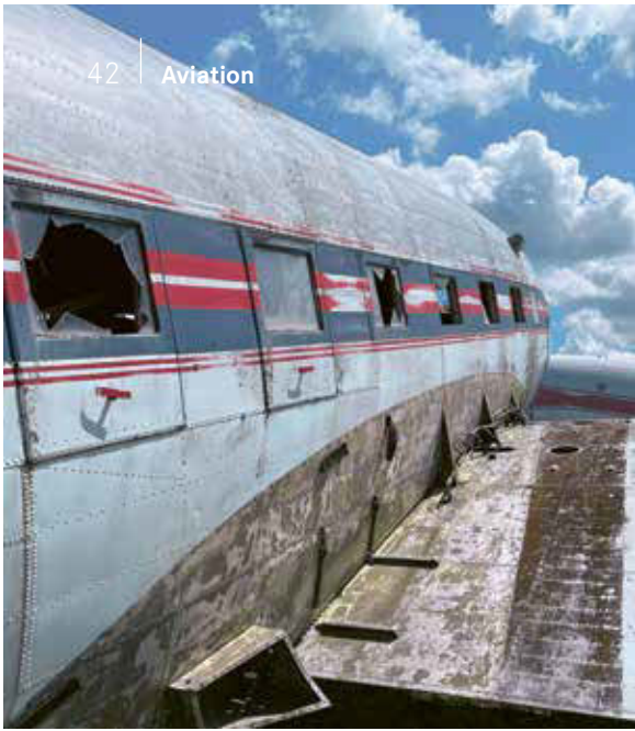
No wings, dents in the fuselage — It's hard to believe that Basler is turning DC-3s that are essentially scrap, some of them 80 years old, back into brand-new aircraft.
