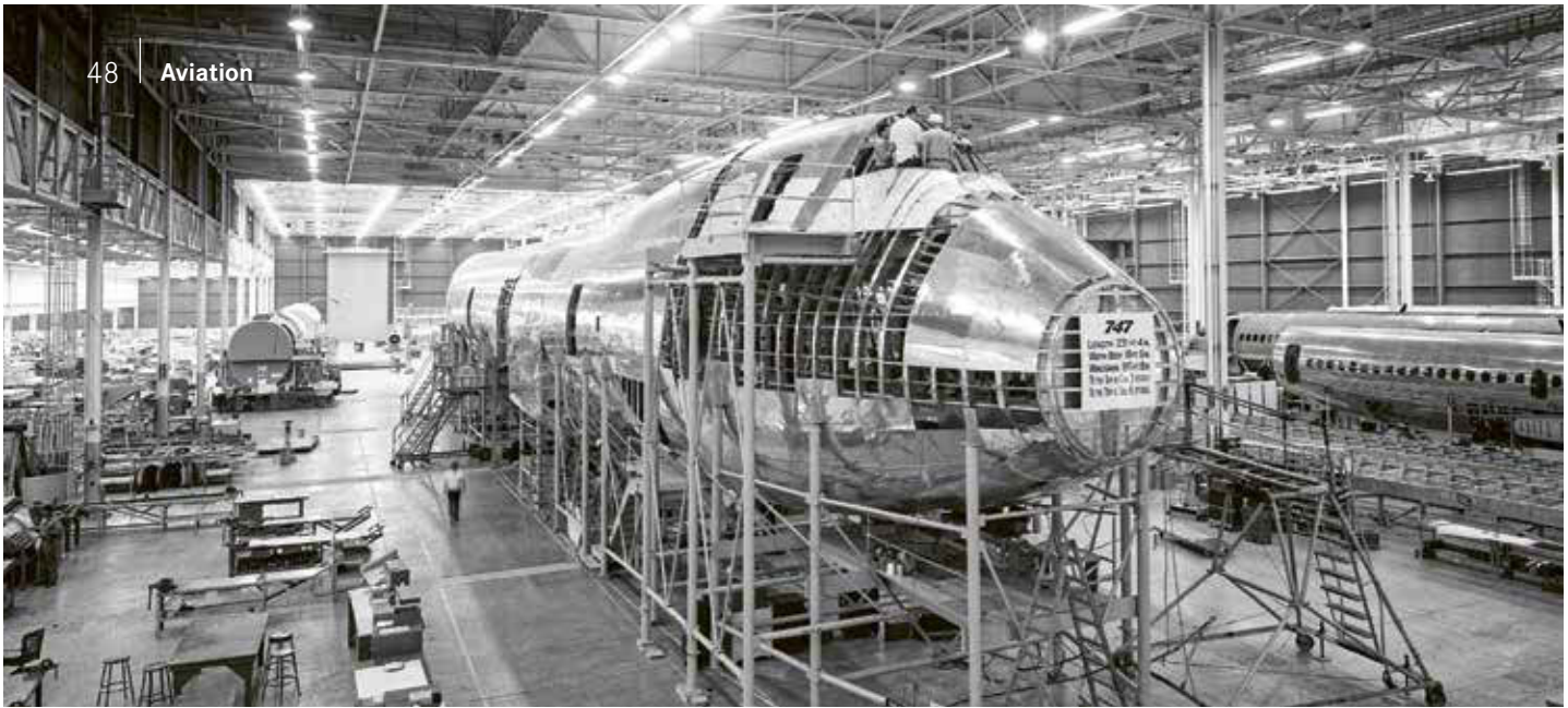
Production facility in Everett — Workers stand in the cockpit area of the full-size 747 mock-up three floors above the ground.
