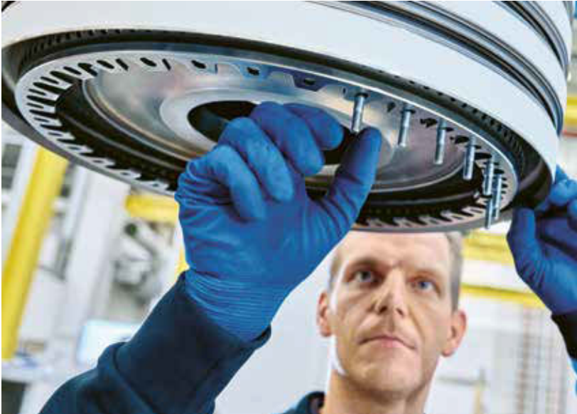
Setup—part 2 — Second, the rear compressor drum is prepared for the tightening process.
