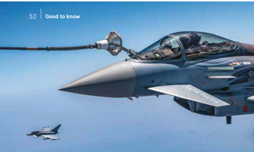
Oversized shuttlecock — In this refueling method, the probe of the aircraft requiring fuel is guided into the drogue.
