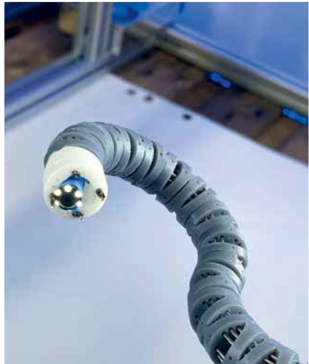
Small and flexible — Cables and leads for the camera and measurement system run through the interior of the miniature robot. The RoBokop will be miniaturized down to a diameter of just six millimeters.
