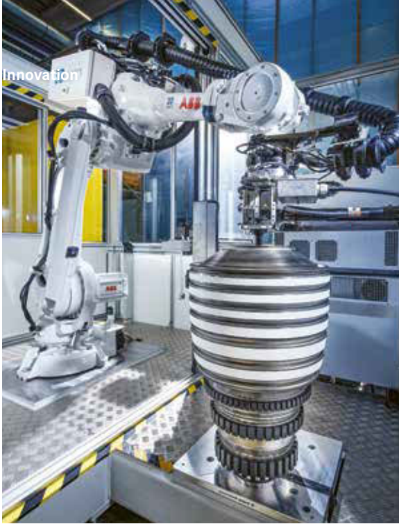
Precision tightening — An industrial robot screws the two rotor drums together—fully automatic and more precise than is possible by human hands.
