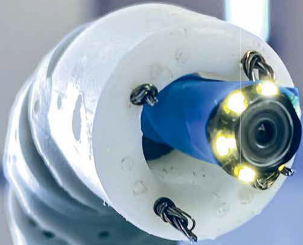
The future of engine repair — A novel continuum robot opens up completely new possibilities in maintenance for detecting hidden damage inside an engine.
