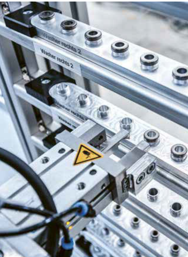
Fully automatic grab — The robot uses a pneumatic grab arm to select the nuts and washers and position them in the flat folding drive.
