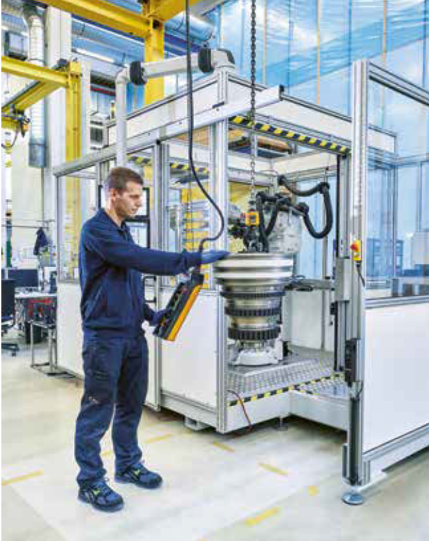
Setup—part 1 — First, the front compressor drum is positioned.
