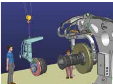
Fourth step — The engine can be disassembled into its individual modules with the help of the smart lifter.
