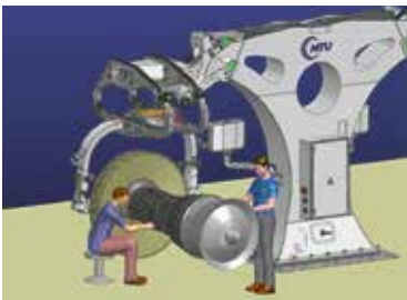
Third step — Mechanics can now adjust the engine's height so they can work on it in an ergonomic position.
