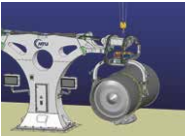
Second step — The overhead crane suspends the engine from its mounting in the FOSng.
