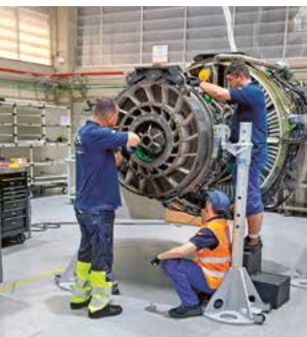
Teamwork — The team from Brazil received support from Ludwigsfelde for the replacement of high-pressure turbine blades on the CFM56-7.
