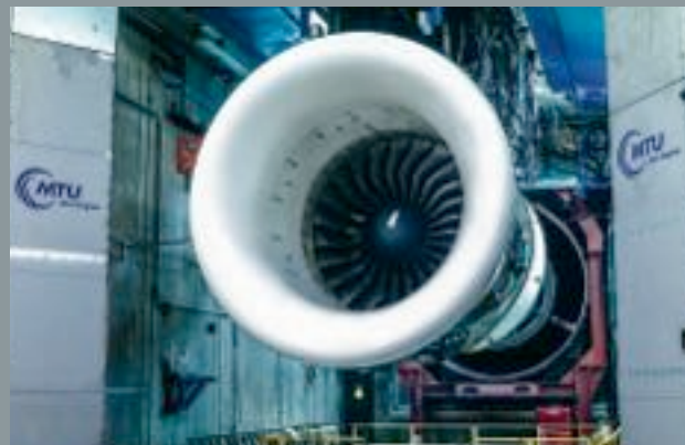
Putting a giant through its paces _____ a GP7000 on a test rig.
