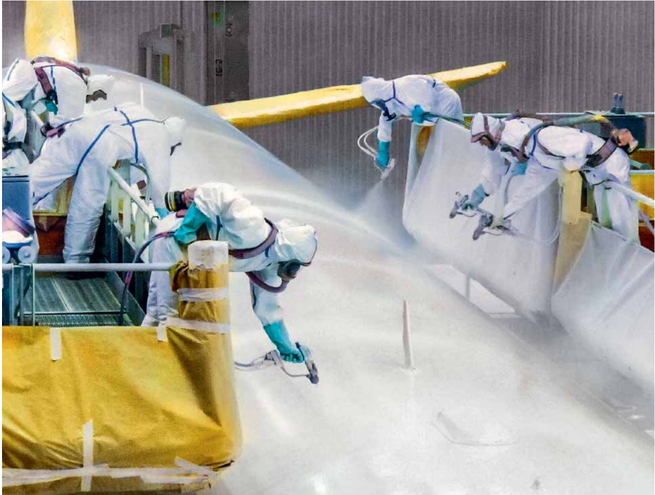
Paint from a gun _____ Among other techniques, Airbus uses electrostatic paint spraying systems, which generate less spray mist. Here the fuselage the first A350XWB for Finnair is painted in Toulouse.
