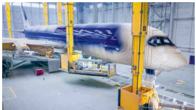
Top coat _____ The aircraft gains color with the third coat of paint—as here at Airbus.
