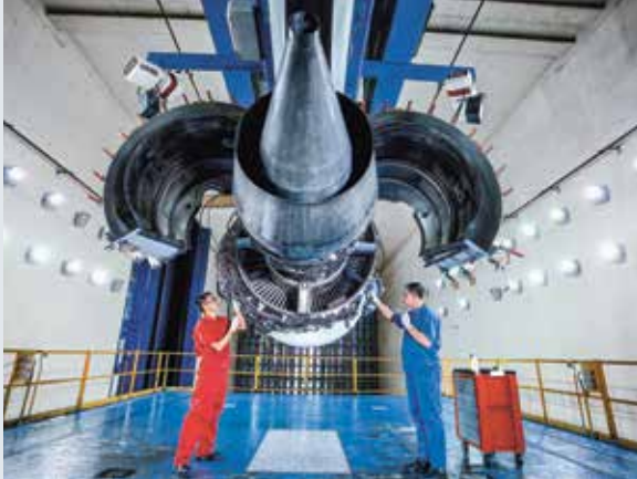
Flexible _____ The test cell at MTU Maintenance Zhuhai is calibrated for the V2500 and for three CFM56 variants.
