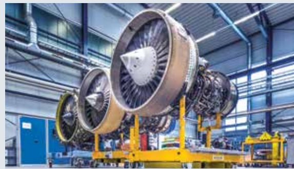
Queuing up — CF34 engines in the test cell rigging shop at MTU Maintenance Berlin-Brandenburg.
