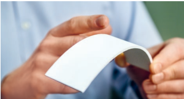
Special properties _____ White CMC cannot be used at temperatures as high as black (SiC/SiC) CMC can, but it doesn't have to be protected from oxygen when exposed to high temperatures.
