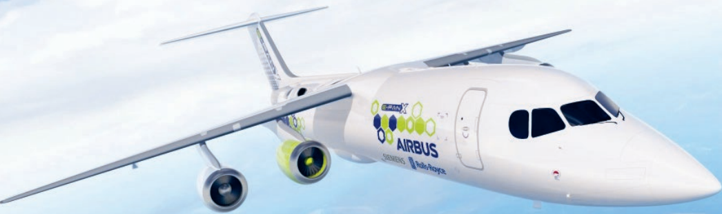
E-Fan X — Initially, just one of this prototype's four engines will be replaced with an electric motor.
