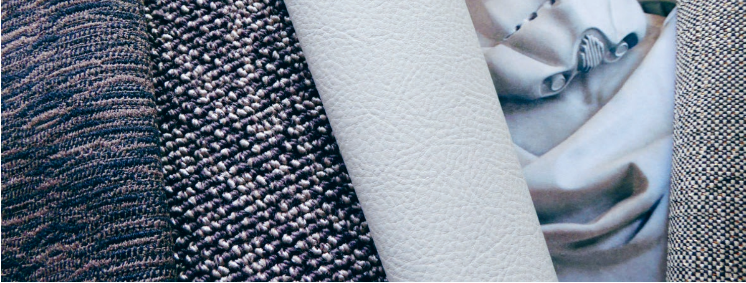
Look and feel ——— Seat covers for aircraft can be made of a wide range of materials, from blended fabrics containing wool, rayon and synthetic fibers to leather. Next to weight, it's a seat cover's look and feel that are the decisive characteristics.
