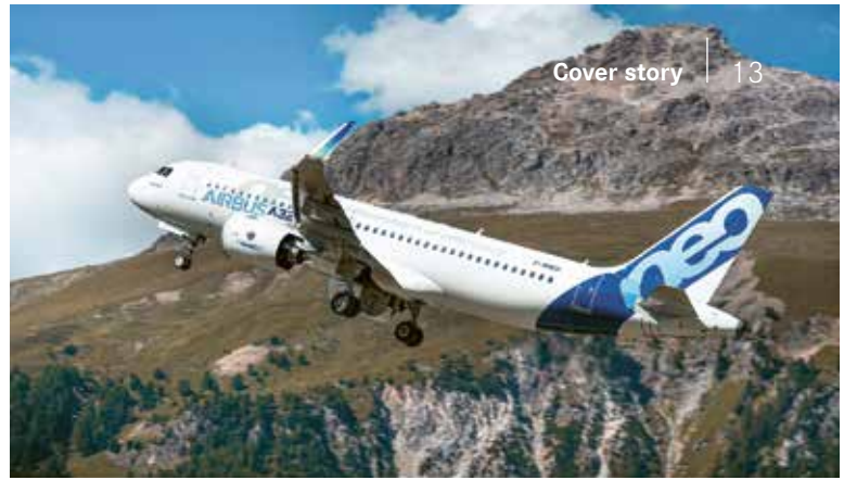
A320neo — The aircraft features new engines and improved aerodynamics. The suffix “neo” stands for “new engine option.”
