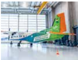
DLR's new research aircraft, "Do 228" D-CEFD — The new DLR research aircraft will be used to test electric propulsion systems.
