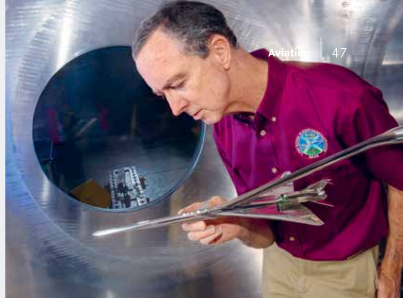
Inspecting a model airplane — Don Durston helped develop a model of NASA's quiet supersonic X-59 aircraft for use in the project's recent wind tunnel tests.
