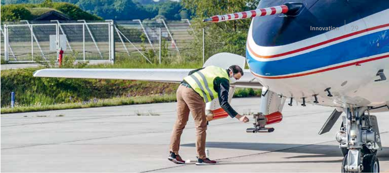
Test of the cloud probe on the Falcon 20E — Prior to a flight of this DLR research aircraft, the cloud probes are tested. These measure physical properties of the ice crystals in the contrail during flight.
