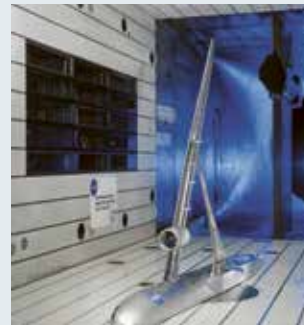
Wide bird ____ A model of the narrow, strutted wing in NASA's Ames Research Center wind tunnel. The wingspan is 44 meters in its original size, which is about 50 percent longer than a conventional commercial aircraft of comparable size.
