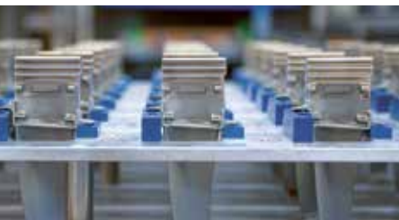
Platinum airfoils — Highly heat-resistant platinum coatings protect against oxidation on, for example, high-pressure turbine airfoils.
