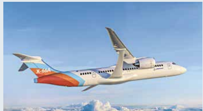
TTBW ____ Since the aircraft is to reach transonic speeds of Mach 0.8 to Mach 1.2 around the sound barrier, the concept is called Transonic Truss-Braced Wing (TTBW).
