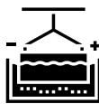
Electroplating — Electroplating is the electrochemical deposition of metallic coatings on objects. The principle behind it was discovered in the 18th century by Luigi Galvani.
