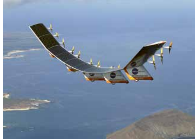
Helios prototype — Developed by NASA, the solar-powered HAP achieved the world record for maximum altitude in 2001, when it stayed at 29,413 meters in the air for 40 minutes.
